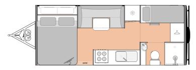
ARE:2500KG T/BALL:120KG HEIGHT:2950MM WIDTH:2500MM LENGTH:7985MM
